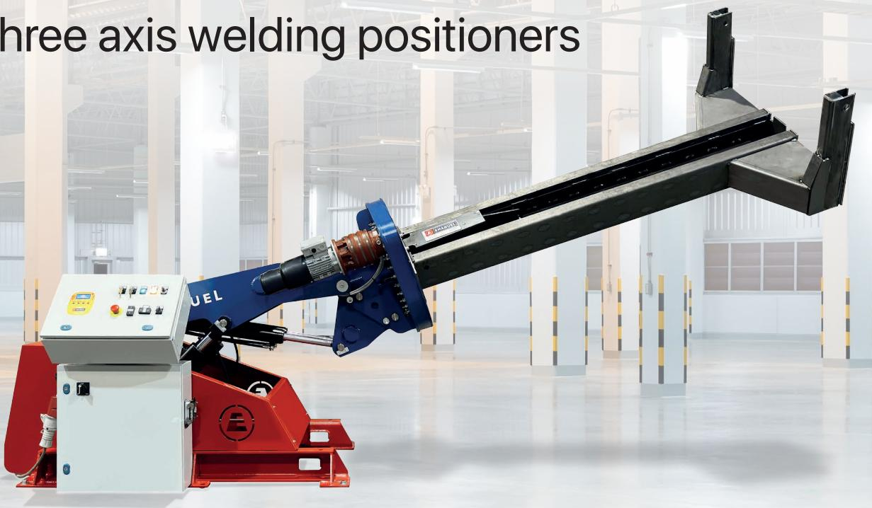
The **WP** is a three axis welding positioner that allows the lifting and the rotation of any work piece during welding and assembly operations. Ergonomic positioners are used during welding and assembly operations of big work pieces that are manufactured by companies of all sectors. The ergonomics, technical characteristics and functional flexibility allow you to increase productivity and efficiency by minimizing the handling of the product on which it is necessary to work on.
